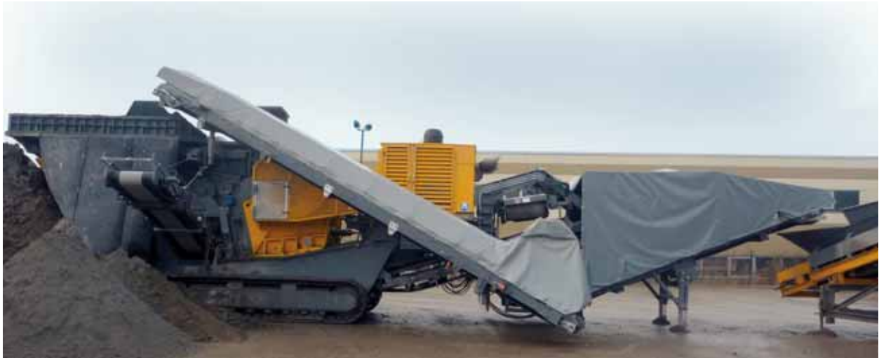
Photo: P1010699_hi.jpg / Text: The Powercrusher PC 1380 J with screenbox HS1 and return conveyor.
